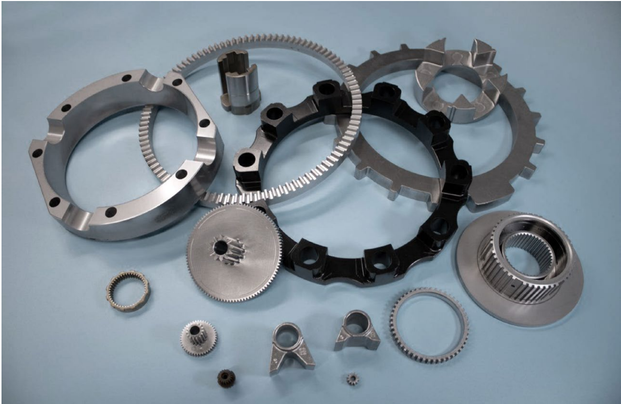
Fig. 11 A selection of automotive components produced by Phoenix Sintered Metals (Courtesy Phoenix Sintered Metals)
