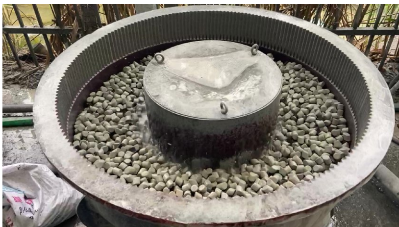
Fig. 3 Sintered Nd 2 Fe 14 B hard magnets undergoing a tumbling process in China (Courtesy Prof David Brown/University of Birmingham [12])
