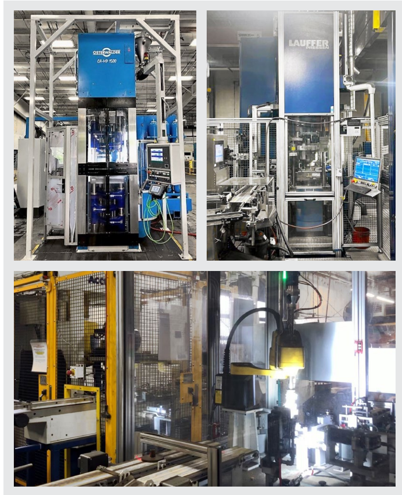
Fig. 8 Upper left and right: metal powder presses at Phoenix Sintered Metals; bottom: a vision/resonance inspection and honing cell (Courtesy Phoenix Sintered Metals)
