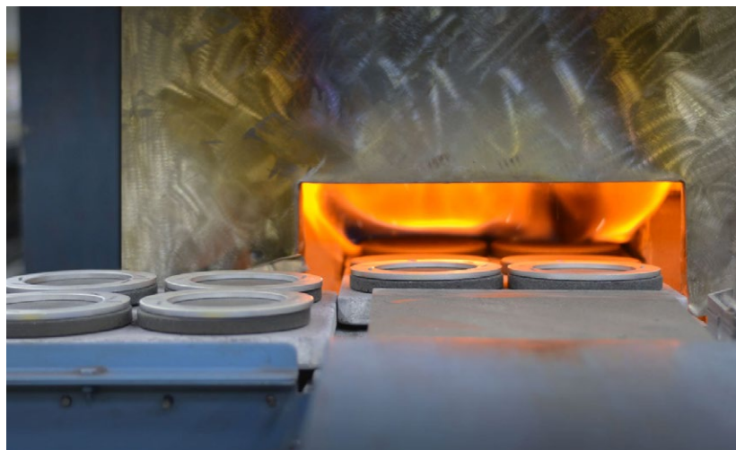
Fig. 1 Parts entering a high-temperature continuous furnace at Phoenix Sintered Metals (Courtesy Phoenix Sintered Metals)
