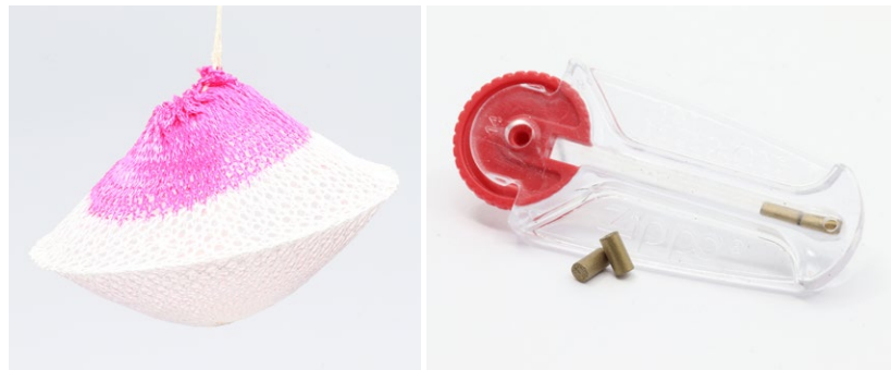
Fig. 1 Two of the first successful technical products containing Rare Earths (RE). Auer's incandescent gas mantle lights (left) initially contained radioactive Th; later, Th was substituted by non-radioactive lanthanoids like Y and Ce. This development shows how closely period 6 and 7 elements are related (in mining and application). Ferrocium flint spark/fire strikers (right) are still made from Auermetall for the Zippo brand by Treibacher Industrie AG. Cerium shows the lowest ignition point of all lanthanoids with \vartheta \approx 165^\circ\text{C} which explains its preferred usage (Courtesy GKN Powder Metallurgy Engineering GmbH)
