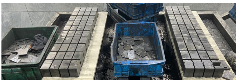
Fig. 4 Sintered Nd 2 Fe 14 B hard magnet blocks sliced by diamond wire saw (Courtesy Prof David Brown/University of Birmingham [12])
