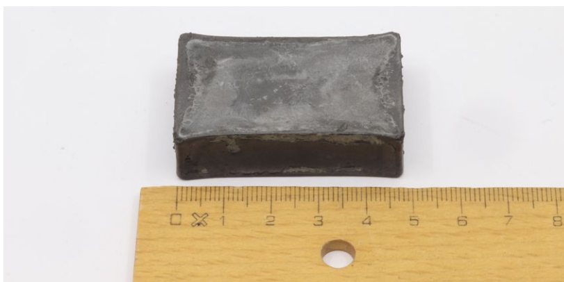
Fig. 6 A sintered Nd 2 Fe 14 B hard magnet block with a certain deviatoric shape deviation, necessitating further machining steps (Courtesy GKN Powder Metallurgy Engineering GmbH)
