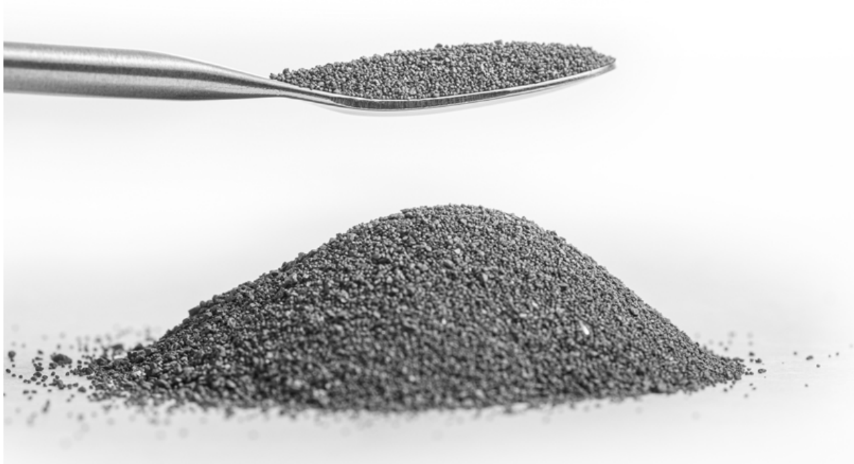
Fig. 4 Recycled titanium metal powders produced by IperionX from 100% scrap feedstock using Hydrogen Assisted Metallurgical Reduction (HAMR) technology and used in the HSPT process (Courtesy IperionX)
