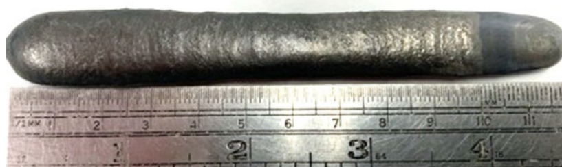
The metal was further refined through distillation, with the resulting metal remelted and formed into a specific shape (Courtesy CMI Hub)
