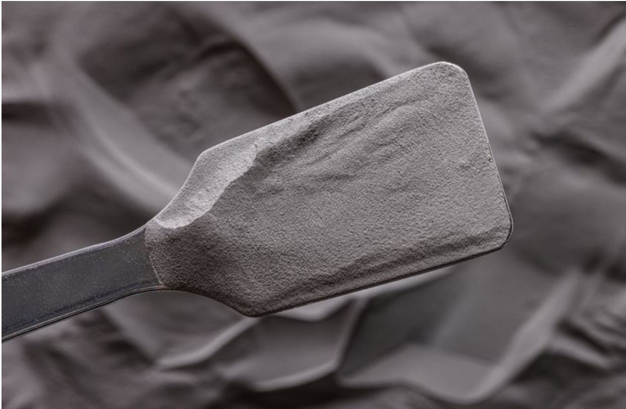
Fig. 7 Spherical Ti-6Al-4V powders are also being developed by IperionX for use in AM and other processes (Courtesy IperionX)
