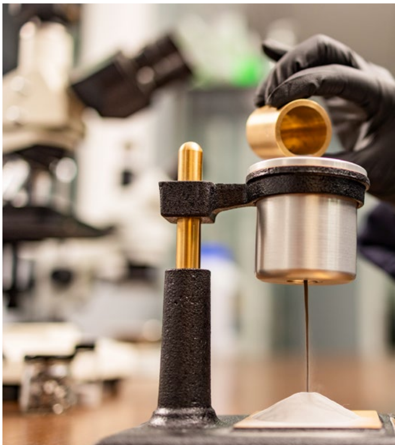
Fig. 6 AM-grade Ti-6Al-4V powder in a flow meter at IperionX (Courtesy IperionX)
