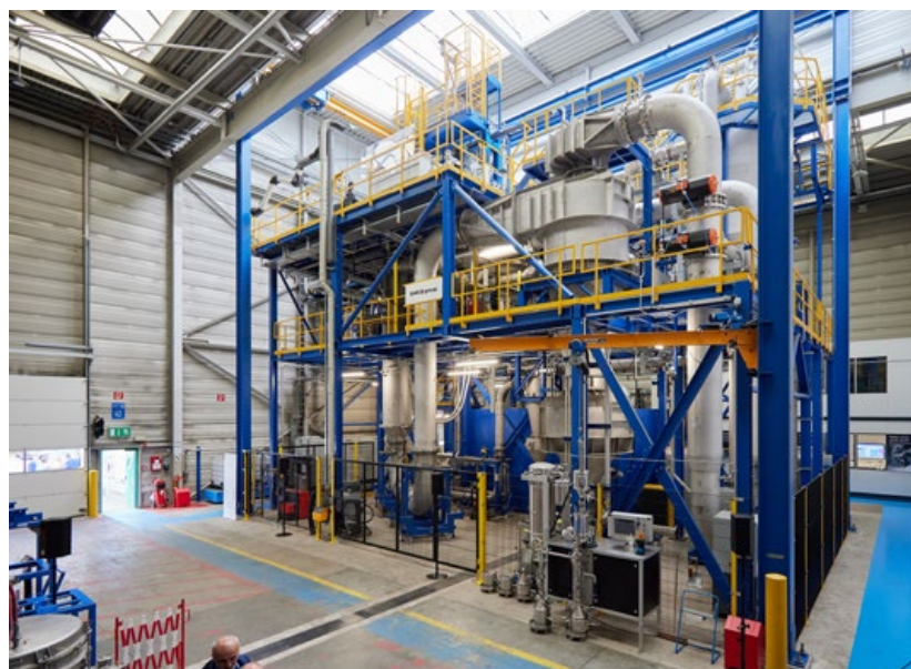
Fig. 1 Outokumpu's vacuum induction/inert gas atomisation (VIGA) metal powder plant at its steel mill in Krefeld, Germany (Courtesy Outokumpu)
