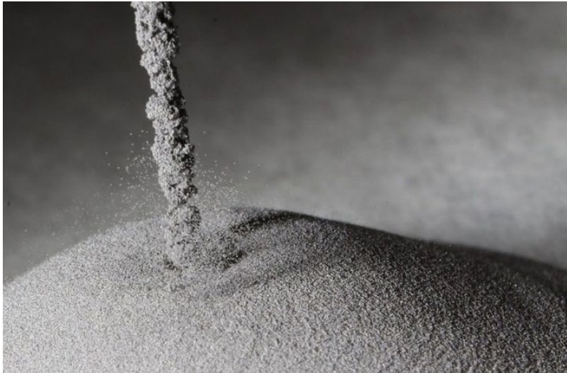
Fig. 4 Plasma atomised titanium powder produced by PyroGenesis Additive (Courtesy PyroGenesis)
