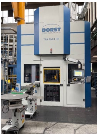
Carbosint has added a new TPA300/4HP hydraulic powder press from Dorst Technologies (Courtesy Carbosint)
