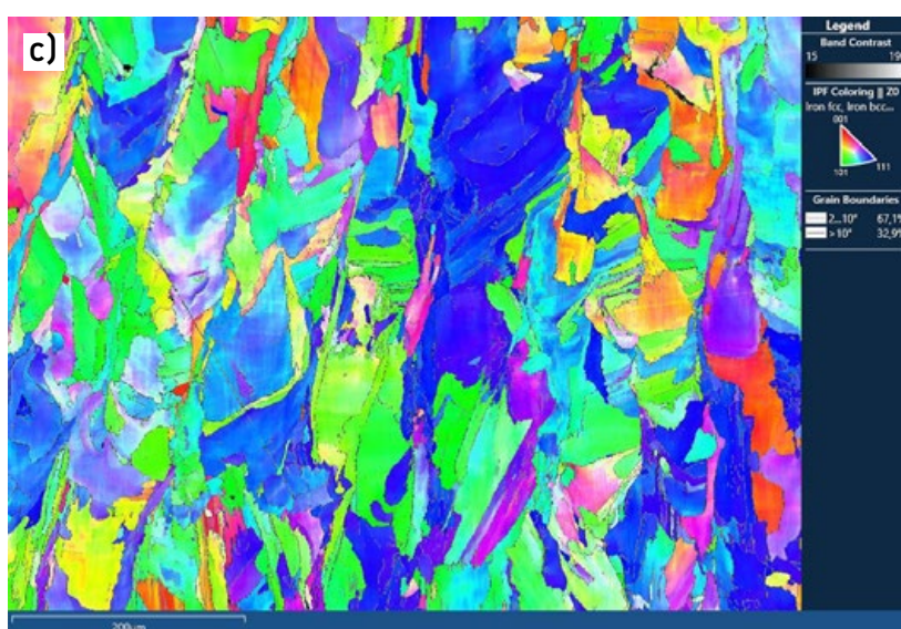
Fig. 10 a) Light optical microscope image of built microstructure b) Scanning electron microscope (SEM) image of single melt pool c) SEM image showing texture of built microstructure. (Figs. 10 b and 10 c: courtesy IEHK Steel Institute, RWTH Aachen University)
